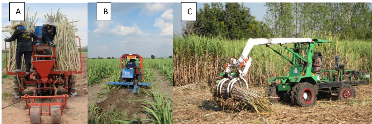
Fig. 2. Mechanization level in sugarcane farming is higher than that of cassava. Fig. 2 (A) Machines are used in planting, Fig. 2 (B) fertilizing and weeding and Fig.2 (C) harvesting
