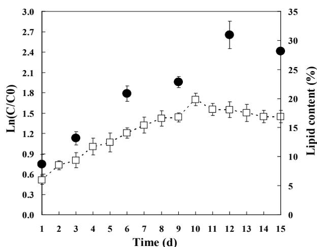
**Figure 2** Specific growth rate and lipid content of isolated *Chlorella* sp. in poultry processing plant effluent LnC/C<sub>0</sub> (open square), lipid content (closed circle)
