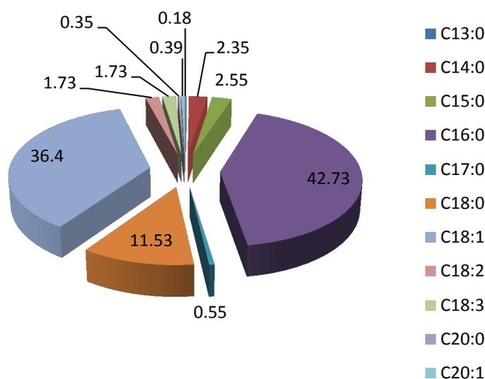
**Figure 3** Fatty acid composition of biodiesel from the isolated *Chlorella* sp. lipid
