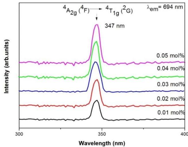
**Figure 4** Luminescence excitation spectra of ZABaB:Cr<sup>3+</sup> glass samples with x = 0.01, 0.02, 0.03, 0.04 and 0.05 mol%
