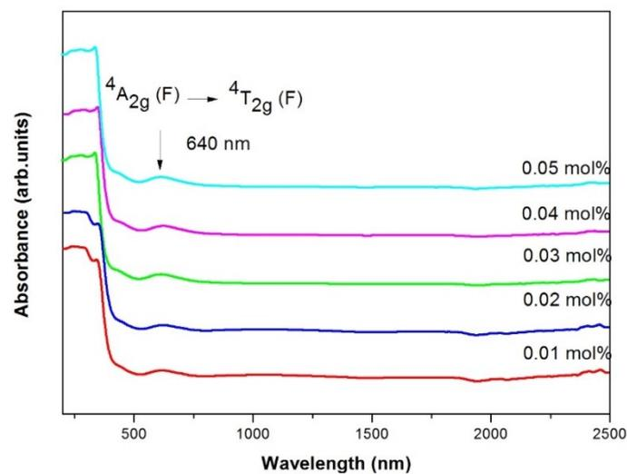
Figure 3 Optical absorption spectra of ZABaB:Cr<sup>3+</sup> glass samples at room temperature
