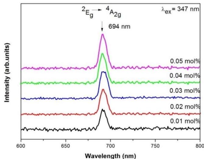
**Figure 5** Luminescence emission spectra of ZABaB:Cr<sup>3+</sup> glass samples with x = 0.01, 0.02, 0.03, 0.04 and 0.05 mol%
