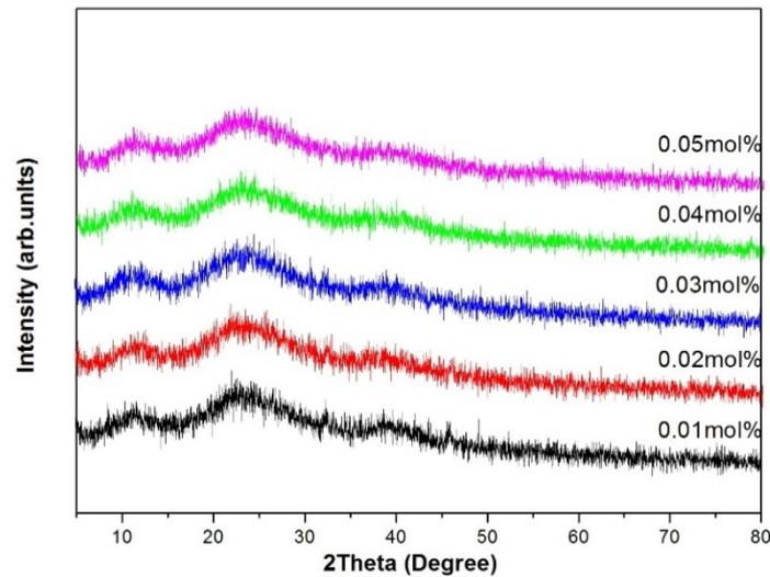
Figure 2 XRD patterns of ZABaB:Cr<sup>3+</sup> glass samples with x = 0.01, 0.02, 0.03, 0.04 and 0.05 mol%
