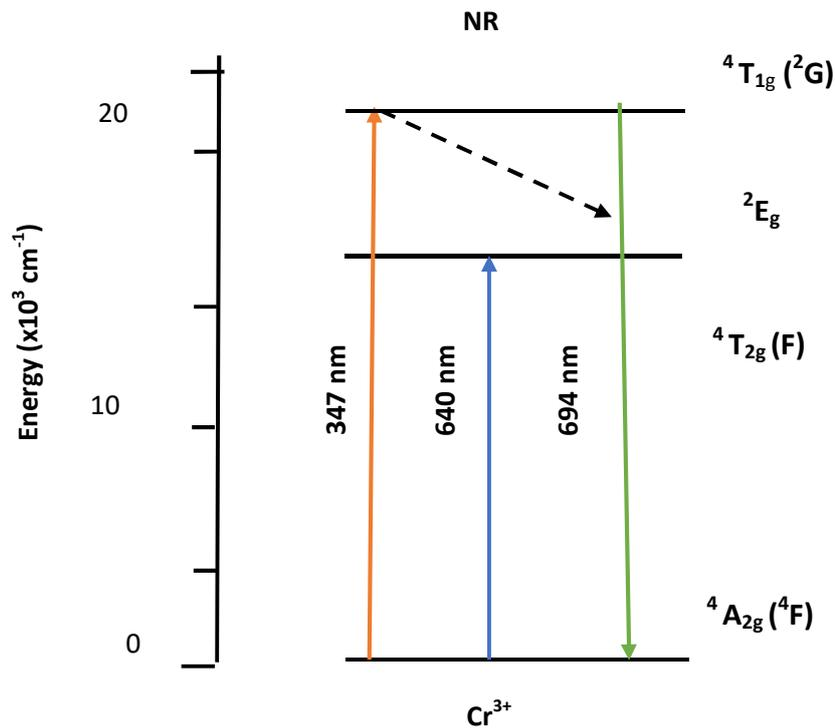
Figure 6 Diagram of partial energy levels of ZABaB:Cr<sup>3+</sup>
