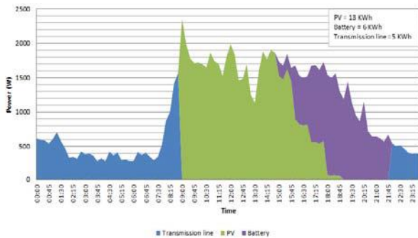
Figure 6 Power consumption in solar home with energy management by the frugal discharge
