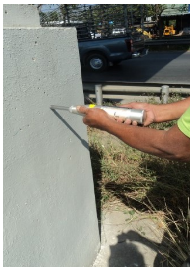
Figure 2 Measurement the reflectance of concrete with Schmidt hammer
