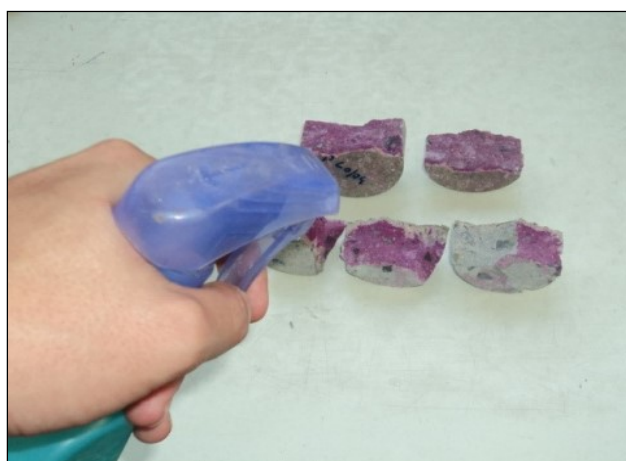
Figure 3 Spraying with a phenolphthalein solution to concrete sample
