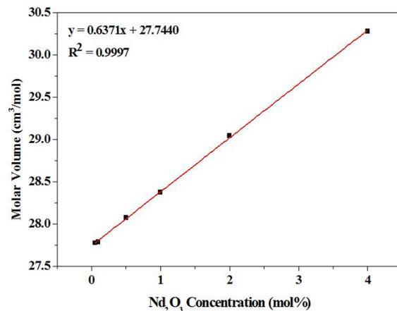
**Figure 2:** The variation of molar volumes as a function of Nd<sub>2</sub>O<sub>3</sub> contents in NBB oxyfluoride glasses.
