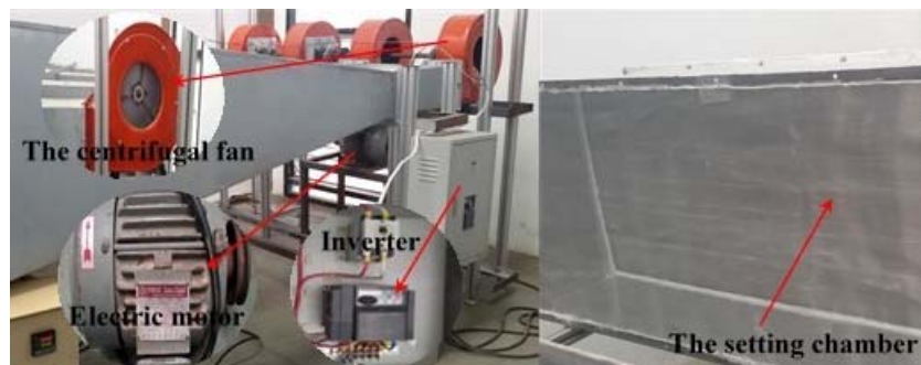
Figure 4 The centrifugal fan, electric motor, inverter and the setting chamber
