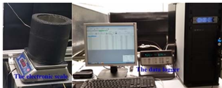
Figure 7 The electronic scale, thermocouples, and humidity probe connected to the data logger.
