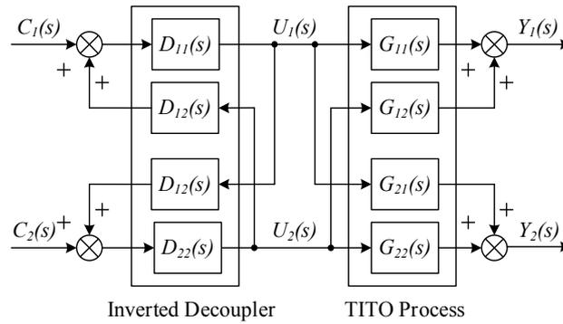
**Figure 1** Inverted decoupling of a TITO process
