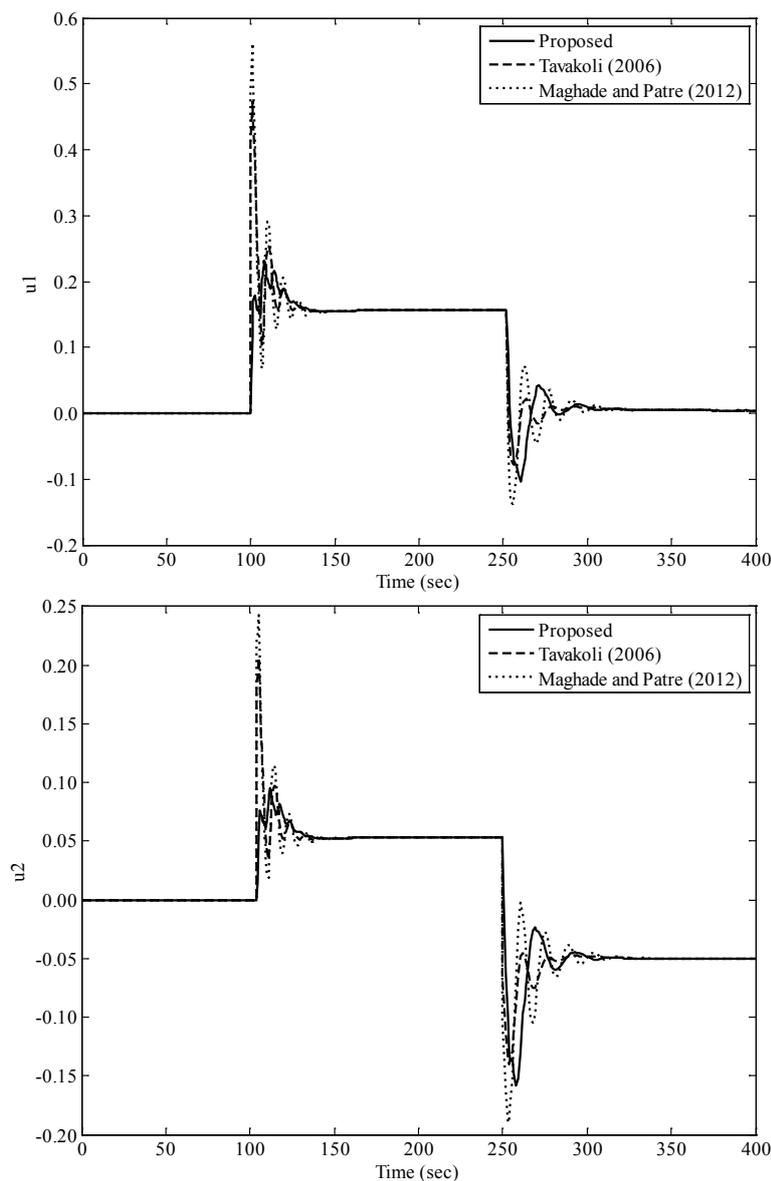
**Figure 5** Control signal response a) the controller 1 ( $u_1$ - $r_1$ ) and b) the controller 2 ( $u_2$ - $r_2$ )
