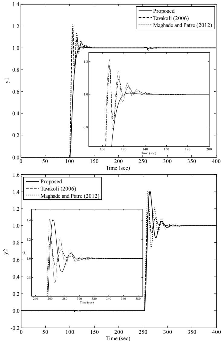
**Figure 4** Unit step response a) the loop-1 ( $y1-r1$ ) and b) the loop-2 ( $y2-r2$ )
