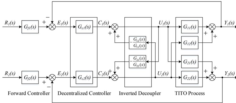
**Figure 3** Decentralized PID controller based on inverted decoupling for TITO system
