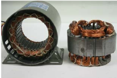
Figure 1 Stator frame and main parameters of prototype motor
