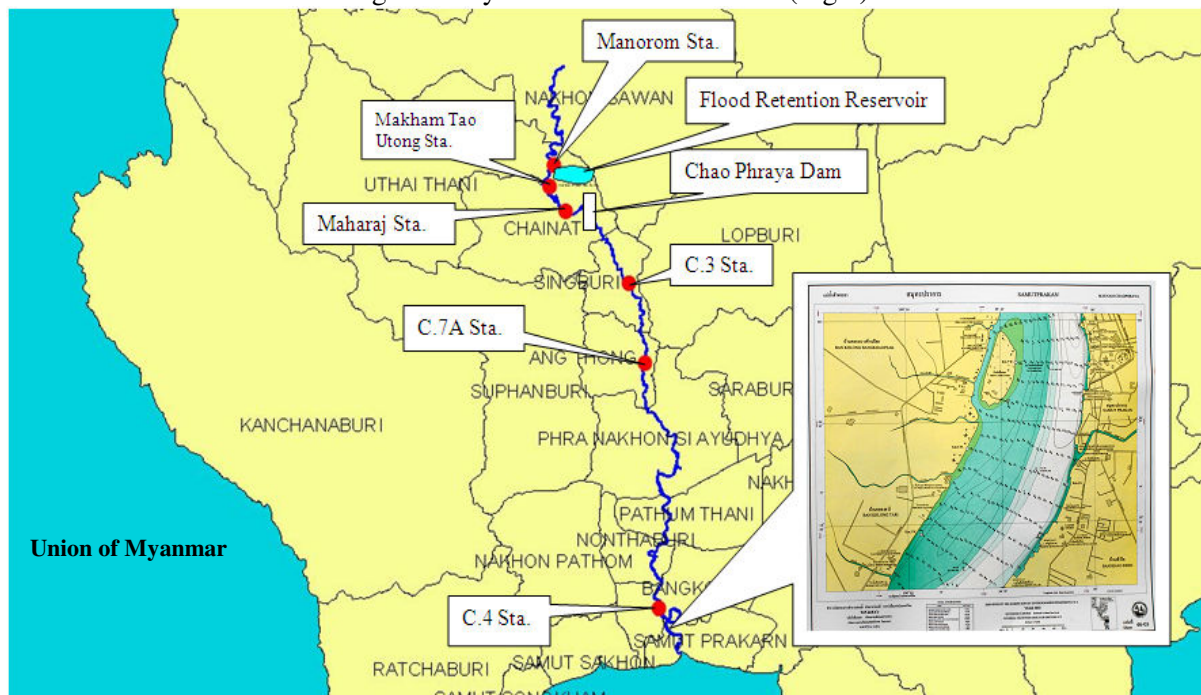
Fig. 3 HEC-RAS model of the lower Chao Phraya river basin with calibration stations and the flood retention/recharge reservoir. The smaller inlet represents a zoomed-in map of a typical river reach that has been used for the preparation of the ArcGis maps and the input data.
